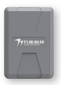
The WER09-01i roadside unit is the core equipment of the gantry end in the ETC segmented billing system. It exchanges information with the OBU or CPC card in DSRC mode, collects the information in the OBU or CPC card, and sends it to the background server in real time.
